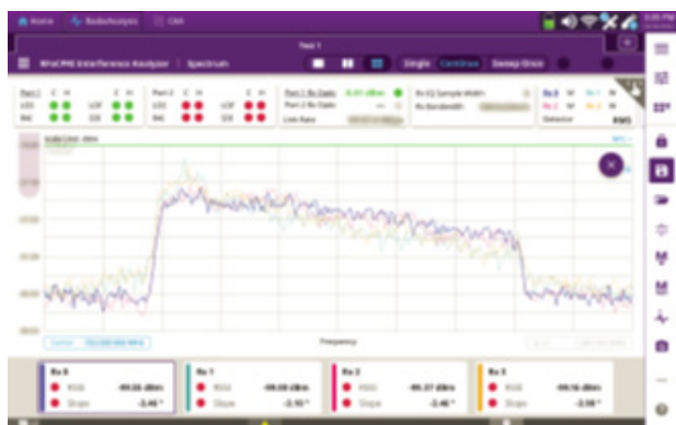
VIAVI OneAdvisor 800 detecting the presence of PIM
