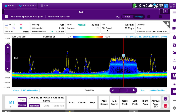
Figure 37: Persistent display showing interference signals in 2.4GHz band.
