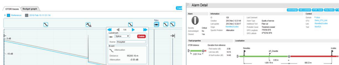
Figure 23: OTDR detailed trace view and SLM view
