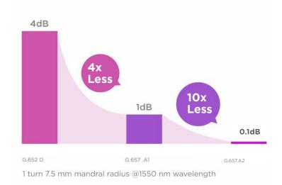
Celesta ribbon cable is made using future-ready G.657.A2 bend insensitive optical fibre and offers industry's lowest attenuation in ribbon cables.
