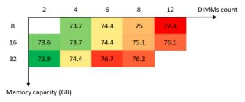
Fig. 7. Idle power consumption (in watts) for different memory configurations (capacity vs DIMM count).
