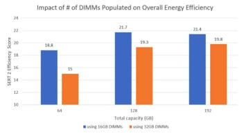
Fig. 6. Impact of # of DIMMs populated on SERT 2 energy efficiency score.
