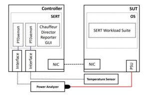
Fig. 3. SERT Environment Setup [15].
