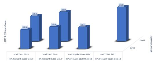
Fig. 9. Energy efficiency score of different servers/CPU and RAM configurations.
