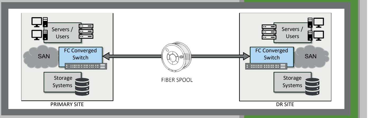
Figure 1: Legacy Fibre Channel distance testing setup which is cumbersome, not flexible or scalable, and limits automated testing
