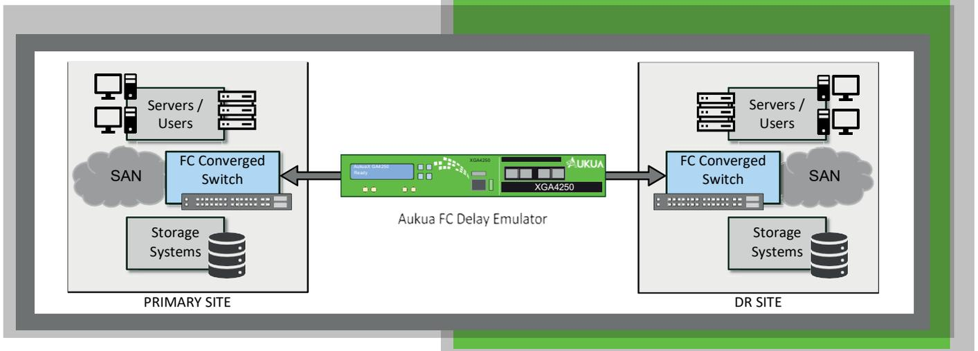
Figure 2: Fibre Channel distance emulation setup with the Aukua FC Delay Emulator
